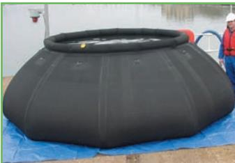
A self-supporting open top storage tank, manufactured from reinforced neoprene-coated fabric, with an air filled collar for extra stability.
