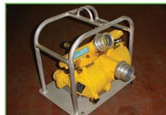
75c hydraulically driven recovered oil transfer pump can be used with the mini and duplex skimmers. The unit is a positive displacement double diaphragm pump mounted in a lightweight two man portable carrying frame. The pump can run dry, will self prime and deliver up to 30m³/hour.
