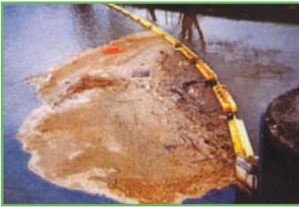
Highly effective range of pollution control barriers designed for permanent deployment in locations where the risk of a spill is on going or for emergency response situations. As well as containing oil, they can also be used as safety barriers or trash/debris containment.
